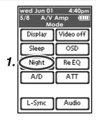
**1.** Tap the **Night** on the remote control unit to turn on the Night mode.
